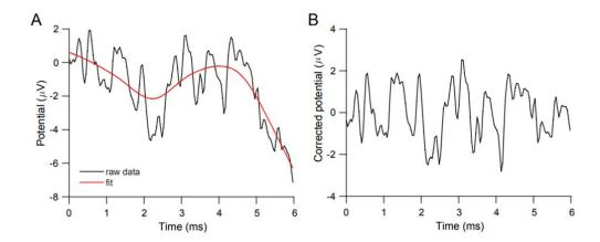
**Suppl. 1.** Baseline correction of single ABR sweep. (A) As an example, raw sweep was fit with a smoothing spline function with a smooth parameter of 0.5. (B) Corrected sweep was obtained by subtracting the fit function from the raw sweep.
