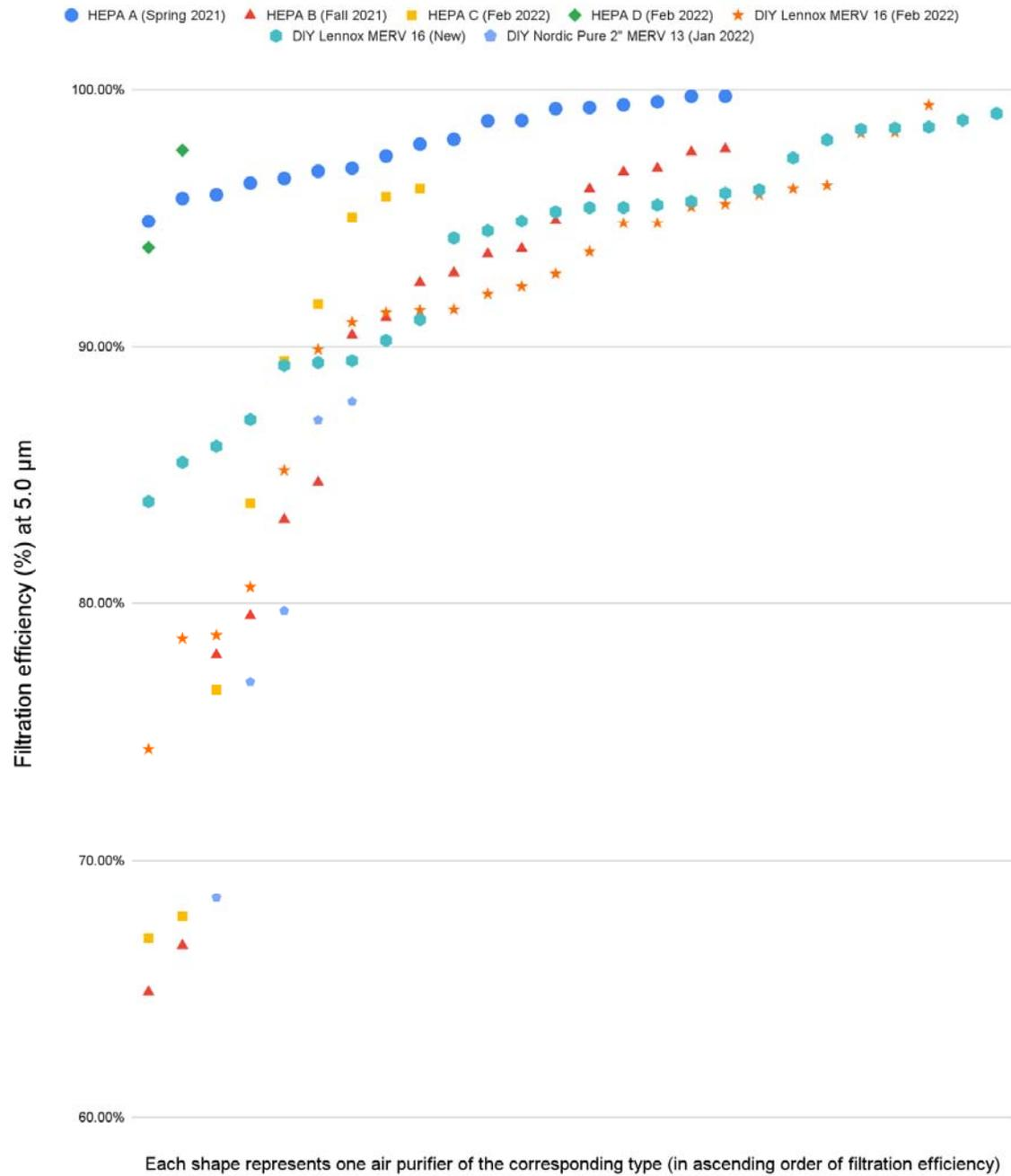
**Figure 6: Filtration efficiency at 5.0  $\mu\text{m}$  of HEPA and DIY air purifiers at the school**
