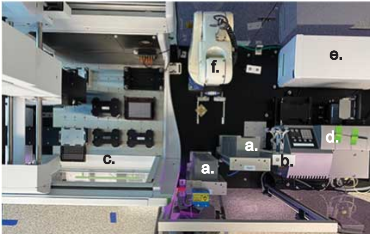
Figure 2. A) Side and B) top views of the ELISA automated workstation consisting of a) Plate hotels, b) suction cup delidder, c) G3 Janus liquid handler, d) washer/dispenser, e) Nivo plate reader, and f) robotic arm.
