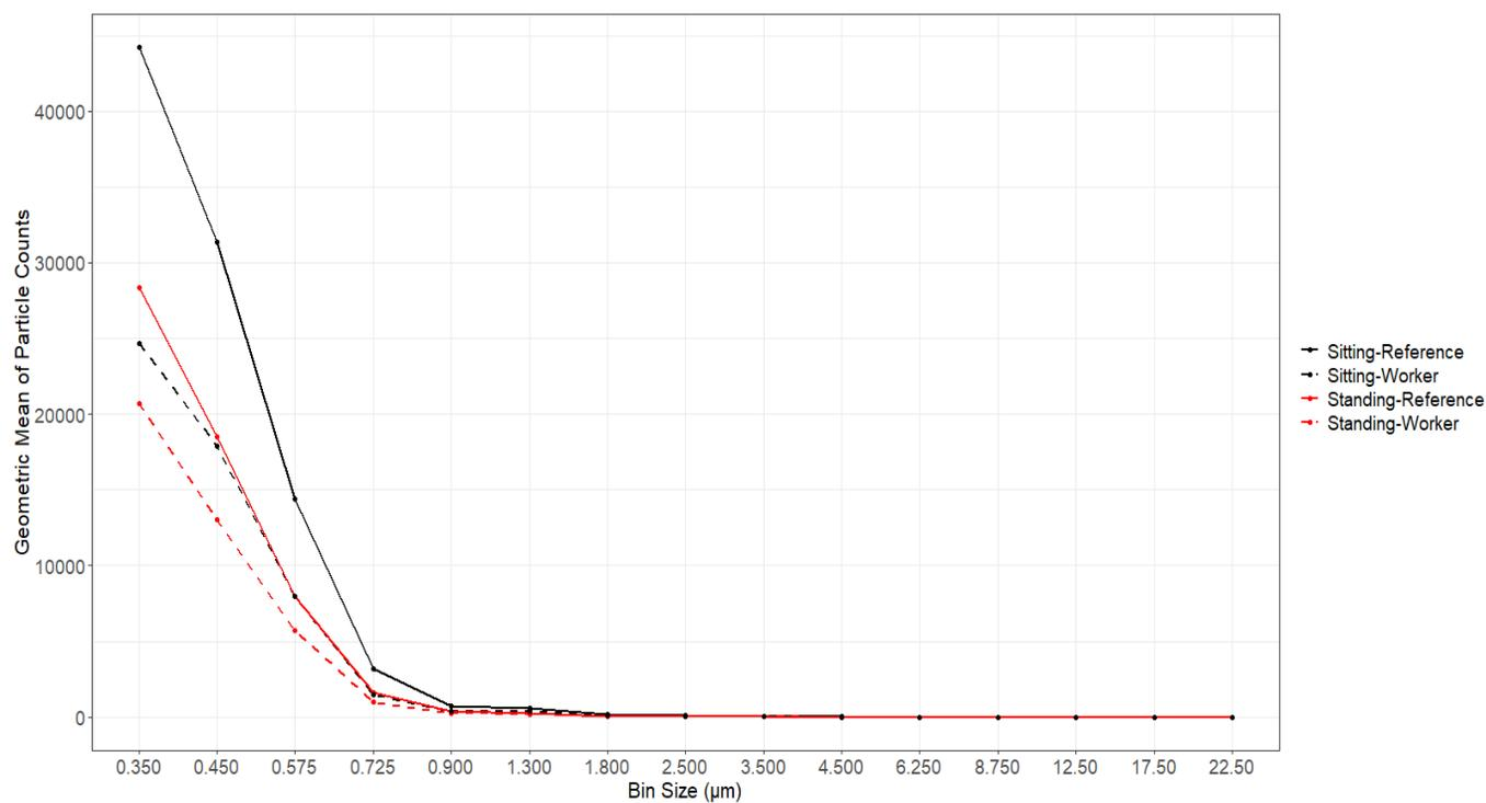
**Figure 4.** Geometric means of particle counts by bin size and OPC location for the configuration of 14 cm (5.5") above cough height and 91 cm (36") width in standing, and 39 cm (15.5") above cough height and 91 cm (36") width in sitting.
