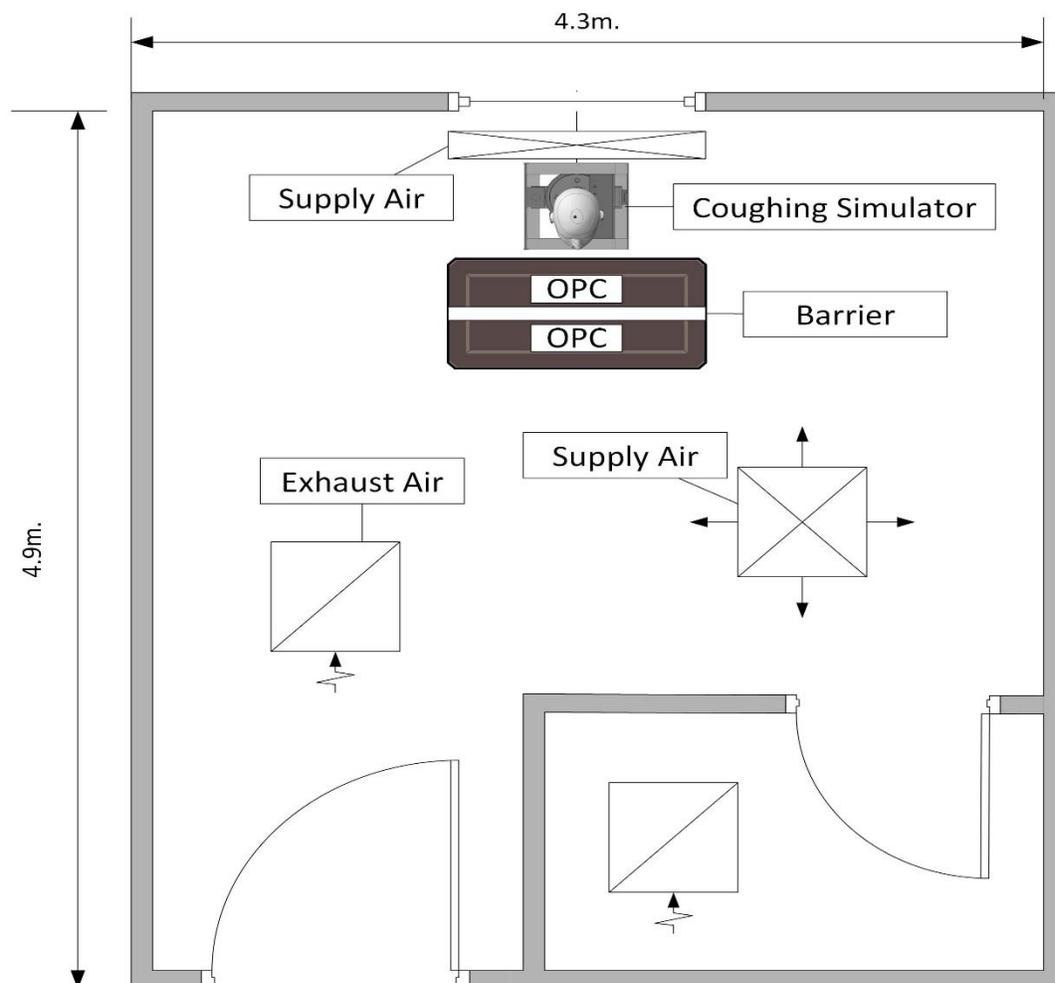
**Figure 1.** Isolation Room 4.9 m (16') long, 4.3 m (14' 2") wide and 2.5 m (8') tall. Note: the exhaust and supply vents were all on the ceiling (2.5 m). The supply closet door was open during the study.
