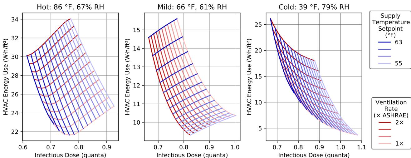
Figure 3: Example tradeoff curves between energy cost and infectious dose for different weather conditions. Values are calculated based on 24 hours of operation for an office, with indicated weather giving average conditions over that span. Each red line holds the ventilation rate constant and varies supply temperature setpoint, while each blue line holds supply temperature setpoint constant and varies ventilation rate.
