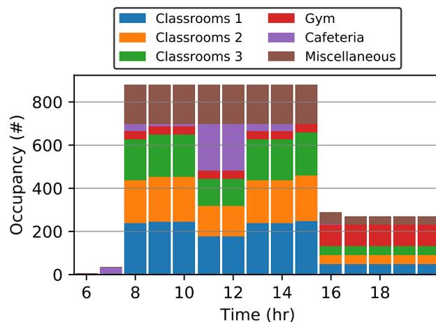
Figure 4: Time-varying occupancy by zone for the school building. Occupancy is zero outside of the indicated time range.
