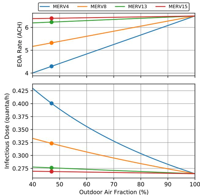
Figure 2: EOA delivery and infectious dose versus outdoor air fraction for various filter types. Results assume 5 ACH total supply flow for the Classroom space type with 1.5 ACH of EOA for the passive physical processes.
