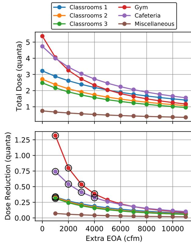
Figure 5: Total dose and reduction in dose for up to eleven in-zone filtration units in each zone of the school. Circled points indicate the eleven locations that have the highest dose reduction, which are thus the optimal locations to place the devices.
