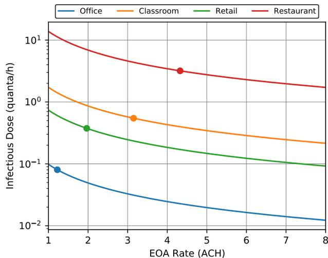
Figure 1: Infectious dose versus EOA delivery for various space types. Indicated points on each curve show the minimum EOA rate expected for each space, which includes the ASHRAE-mandated minimum ventilation plus an additional 0.8 ACH corresponding to the passive physical processes.
