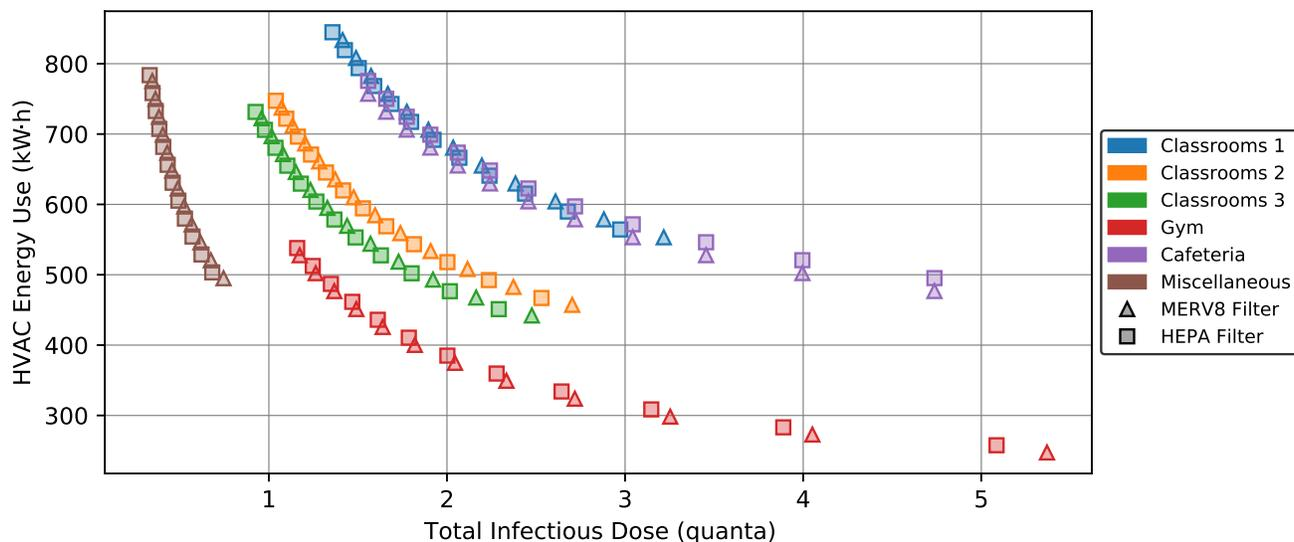
Figure 6: HVAC energy consumption and total dose for each zone assuming up to eleven in-zone disinfection devices for two different in-duct filter types. The rightmost points for each zone correspond to no in-zone devices, while the leftmost points show the effects of all eleven devices.
