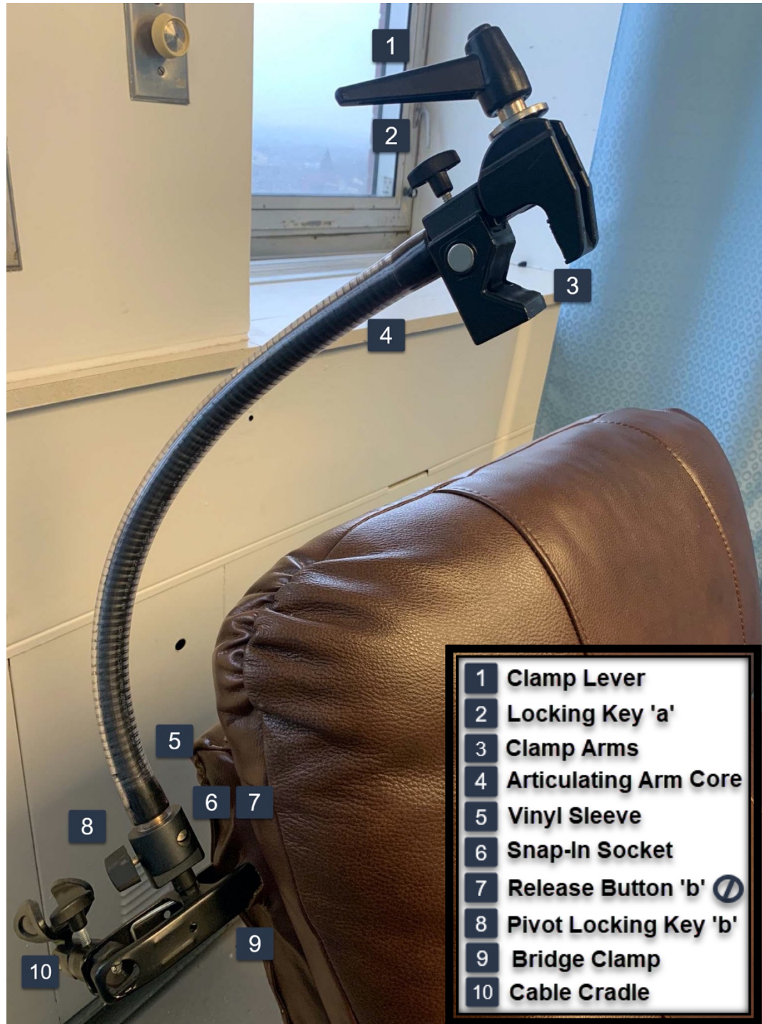
Figure 2: Anchored Articulating Arm (AAA) schematic - AAAs are made out of inexpensive camera tripod equipment and are anchored at their base to the corner of the treatment chair. Coils are held securely by a clamp locking it to the AAA, maintaining position until treatment has been completed, at which time they can be quickly twisted out of the way.
