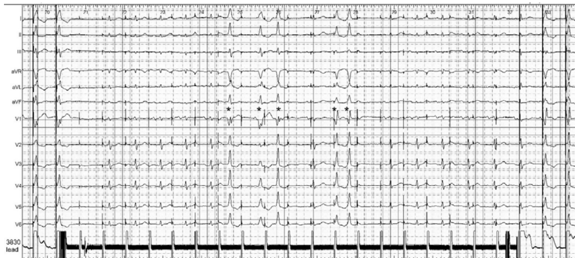
Figure 1. A shower of fixation beats (marked with asterisks) during a single episode of 3830 lead rotation for deep septal lead placement. During rotation, the lead was disengaged from the alligator clip connection to the external pacemaker (marked with the appearance of the noise signal on the 3830 lead channel) for 12 seconds. The first three fixation beats were classified as ‘deep septal fixation beats’ while the last two, of qR morphology, as ‘LBB area fixation beats’. The fixation beats showed progressive change of QRS morphology that is compatible with progressively deeper origin within the interventricular septum. Please note, that the paced QRS morphology when the lead was reconnected with the alligator clip/external pacemaker is nearly identical as the last LBB area fixation beat, while the first fixation beat morphology is nearly identical as the initial paced QRS that served to identify the optimal site for lead advancement. These observations indicate that the fixation beat morphology reflect the actual position of the screw-in electrode helix. LBB – left bundle branch.
