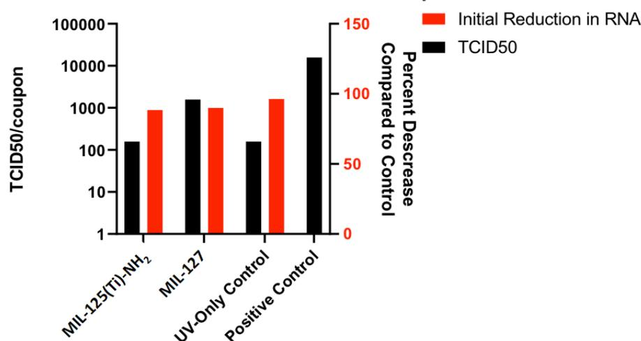
Figure 1. PCR and TCID50 test results showing SARS-CoV-2 Inactivation Coupon treated with MIL-125(Ti)-NH<sub>2</sub> demonstrates greater inactivation (by TCID50) when exposed to UV-C radiation than MIL-127(Fe), although reduction in RNA is identical, indicating RNA damage is not the primary means of inactivation.
