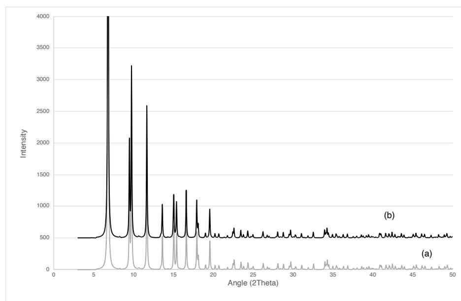
Figure 3. PXRD patterns of a) calculated MIL-125(Ti)-NH<sub>2</sub> and b) experimental MIL-125(Ti)-NH<sub>2</sub>
