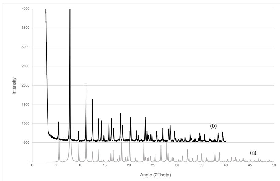
Figure 5. PXRD patterns of a) calculated MIL-127(Fe) and b) experimental MIL-127(Fe)
