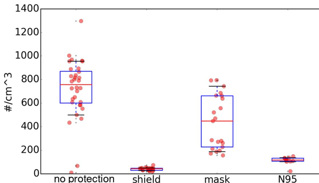
**Fig 4: Total maximal particles number, measured by an APS instrument, comparing un-protected scenario, plastic shield, medical mask and an N95 mask. The horizontal red line marks the median, the blue square indicates the second and third quarter, and the extreme horizontal lines describe the first and ninth decile. Individual values are depicted by red circles.**
