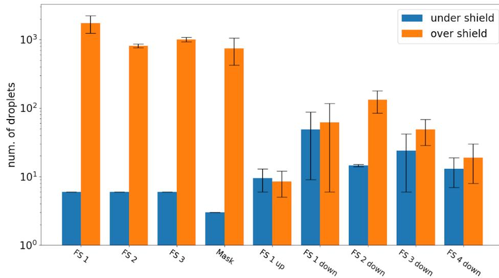
**Fig 5: Overall number of droplets (logarithmic scale) over and under the face shield (FS), for different kinds of shields (FS 1 to 4), a medical mask and different configurations ‘up’ and ‘down’ refer to cases in which a vertical distance was introduced, where in the former, the breathing simulator was positioned 30 cm above the cough simulator and the opposite for the latter. For all repetitions a horizontal distance of 60 cm was kept.**
