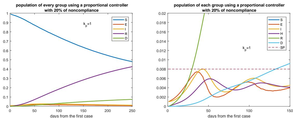
Figure 11: Evolution of every group over time with a proportional control action with gain  $k_p = 1$  (left) and considering 20% of noncompliance of the NPIs policies on average. The picture at the right is a zoom of that at the left. Set point equal to 0.008.
