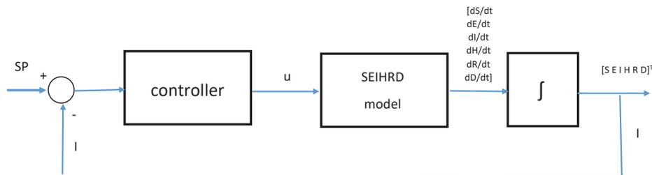
Figure 2: Block diagram of the closed loop control system.
