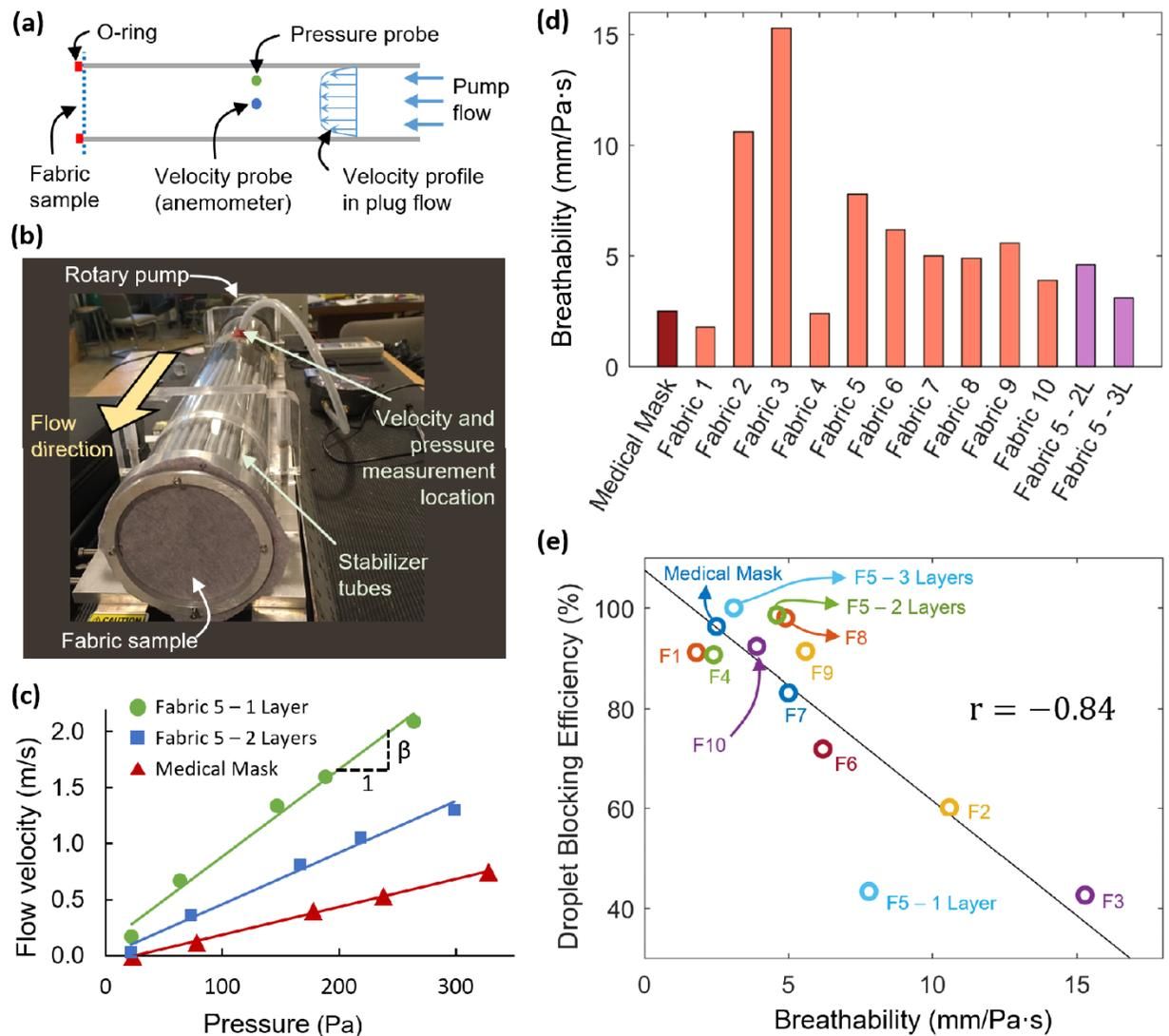
**Figure 3. Measuring breathability.** (a) Schematic illustration of experimental method and (b) image of plug flow tube set-up. (c) Flow velocity vs. pressure plots for selected samples. (d) Breathability measurement results for all samples. (e) Droplet blocking efficiency vs. breathability plot with a regression line illustrating strong negative correlation.
