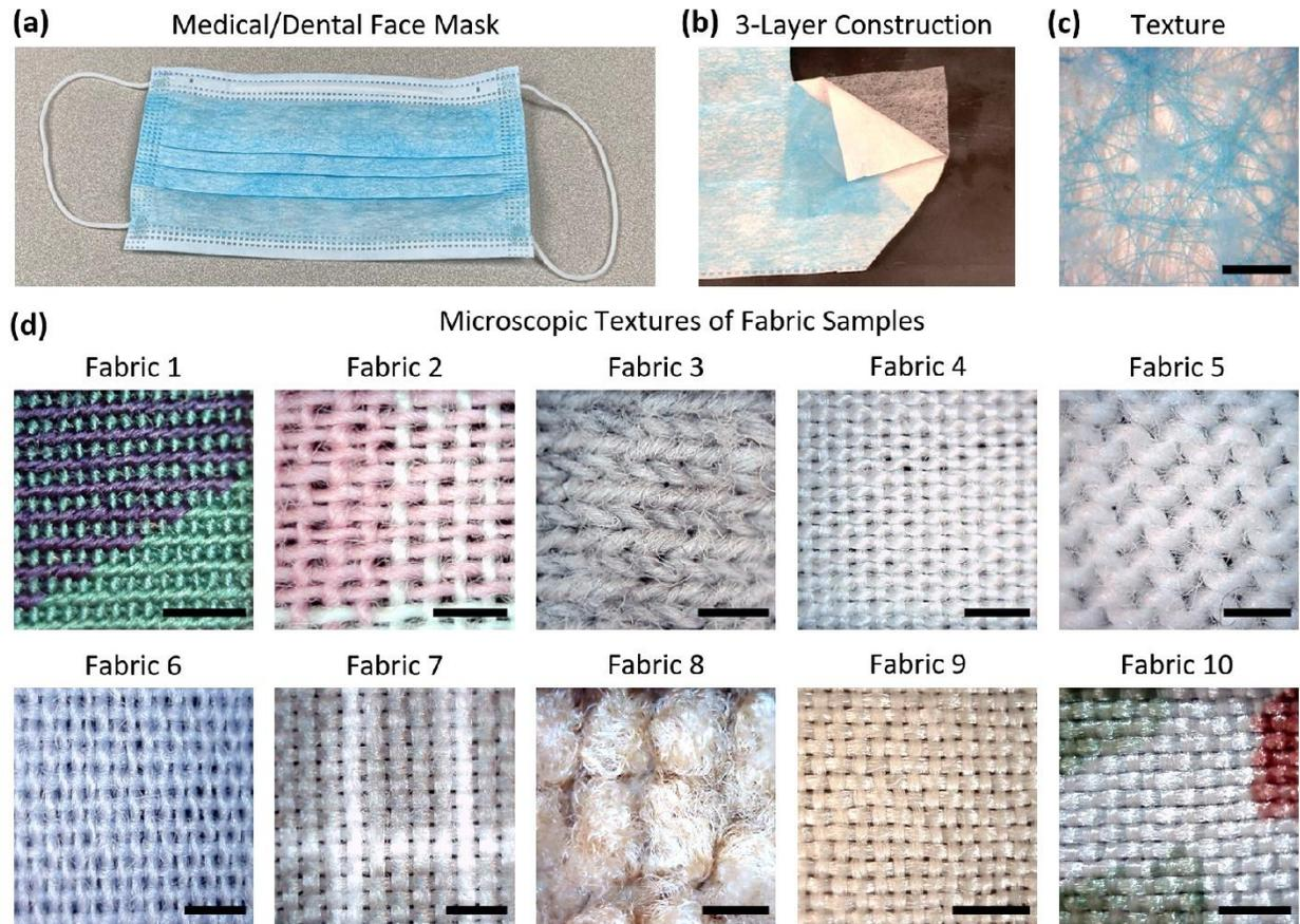
**Figure 1. Samples used in this study.** (a) Image of a medical/dental quality FM-EL style face mask with (b) 3-layer construction, which was used as a benchmark. (c) Microscopic texture of the outer surface of the medical mask. (d) Microscopic textures of the 10 different home fabric samples. All scale bars: 1mm.
