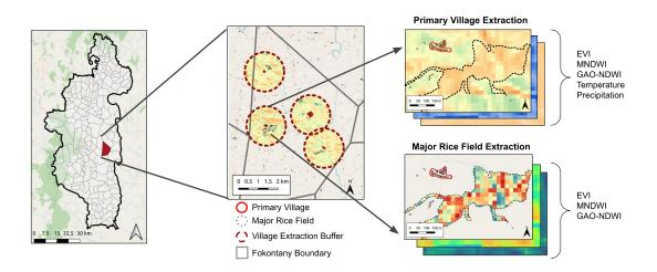
Figure 2. Process of extracting environmental indicators at a fine-scale from satellite imagery for major village and rice field extraction zones. Indicators at the primary village level are extracted using a 1km buffer surrounding the village (red-dashed line), while indicators at the rice field level are extracted within the boundaries of the major rice fields (black dashed line).
