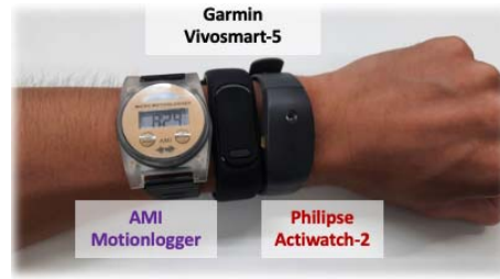
Figure 5. Motionlogger, Actiwatch-2, and Vivosmart-5 on the participant's right wrist during sleep.
