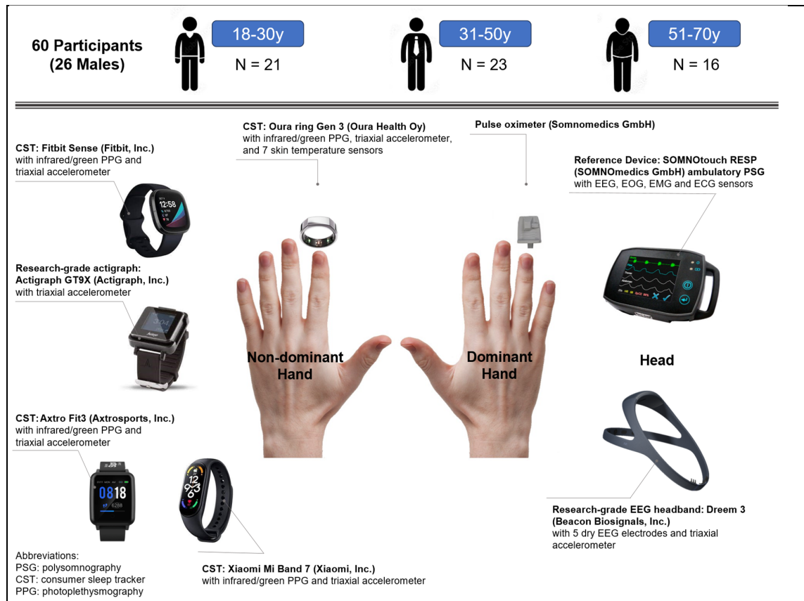
Figure 1. Sample demographics, device placement for a right-handed participant, devices used in the study and their sensors.
