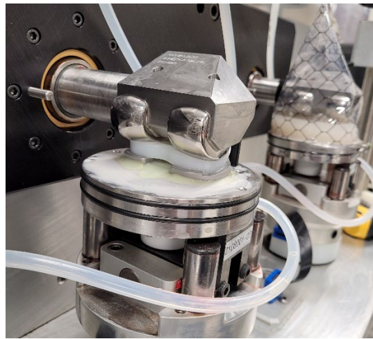
Figure 1. Wear test specimens consisting of PE inlay, tibial, and femoral components fixed in the bench test setup in dry (foreground) and sealed with lubricant (background) state.
