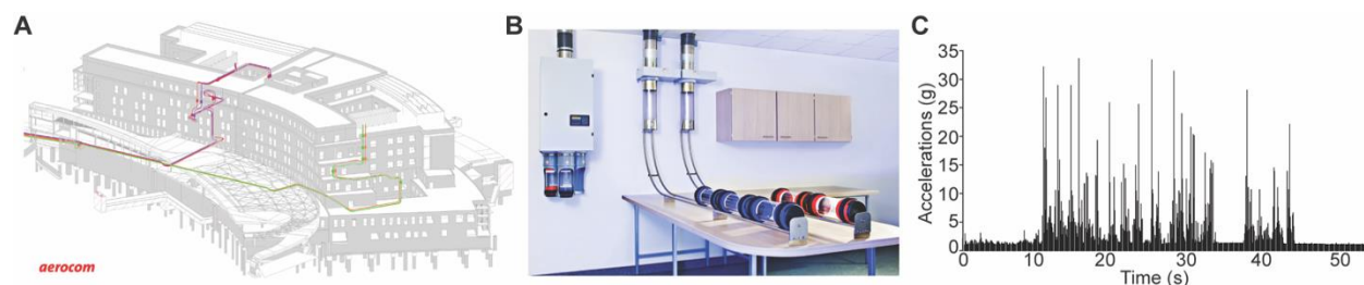
4 5 Figure 1. Characterization of the pneumatic transportation system (PTS). A. Map of the PTS 6 at the Institut de Cancérologie Strasbourg Europe. In red the one used for this study. B. 7 Representation of the setup used for transportation of the monoclonal antibodies (mAbs). C. 8 Characterization of the cumulative (x, y, and z axis) acceleration forces applied to the mAbs.
