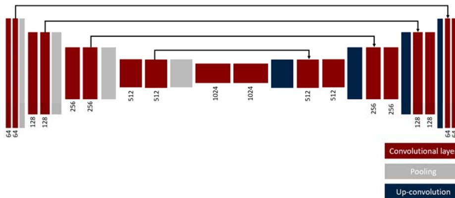
**Figure 3.** The UNet architecture consists of a multiple down-sampling (left) and up-sampling blocks (right). Each block consists of a set of convolutional units, where each unit consists of a sequence convolution, batch normalization, and non-linear activation (ReLU).
