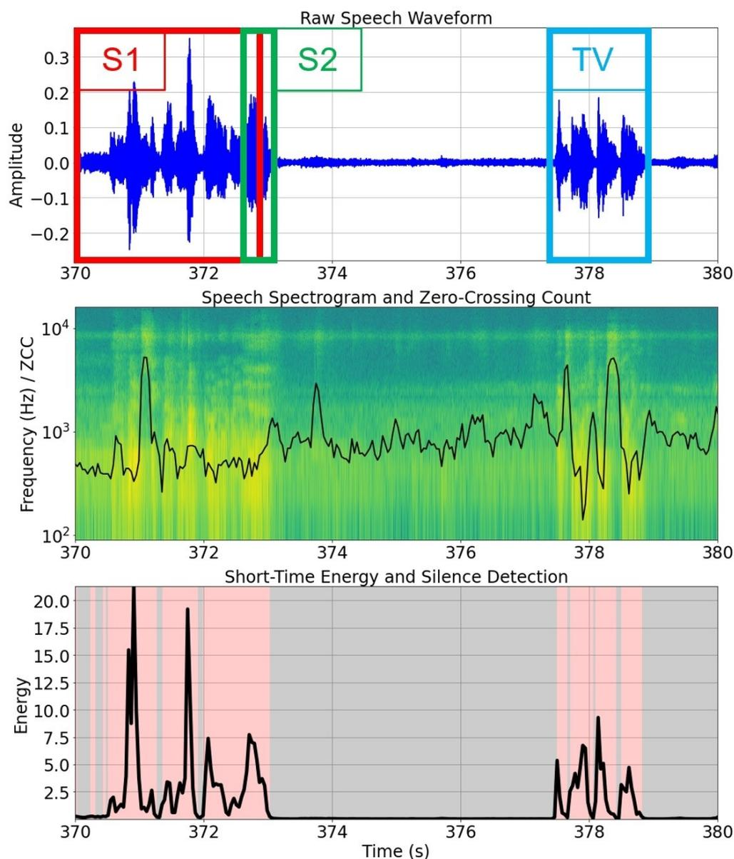
**Figure 2.** TV task speech pre-processing for speaker diarisation. *Top*, raw speech waveform with overlapping speakers 1 and 2 labelled, as well as the TV. *Middle*, speech spectrogram with zero-crossing count, a feature useful for detecting voiced and unvoiced speech, overlaid. *Bottom*, silence removal using a naïve energy detector after careful denoising.
