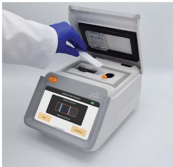
Gazelle device with lateral flow immunoassay
