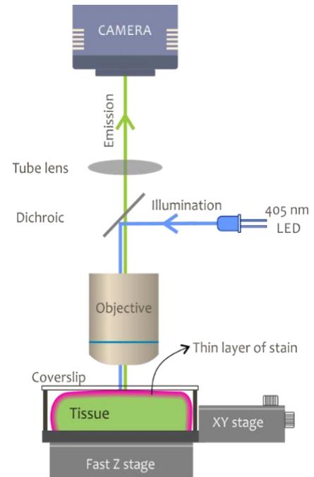
Fig. 2. Schematic design of a FIBI imaging microscope.
