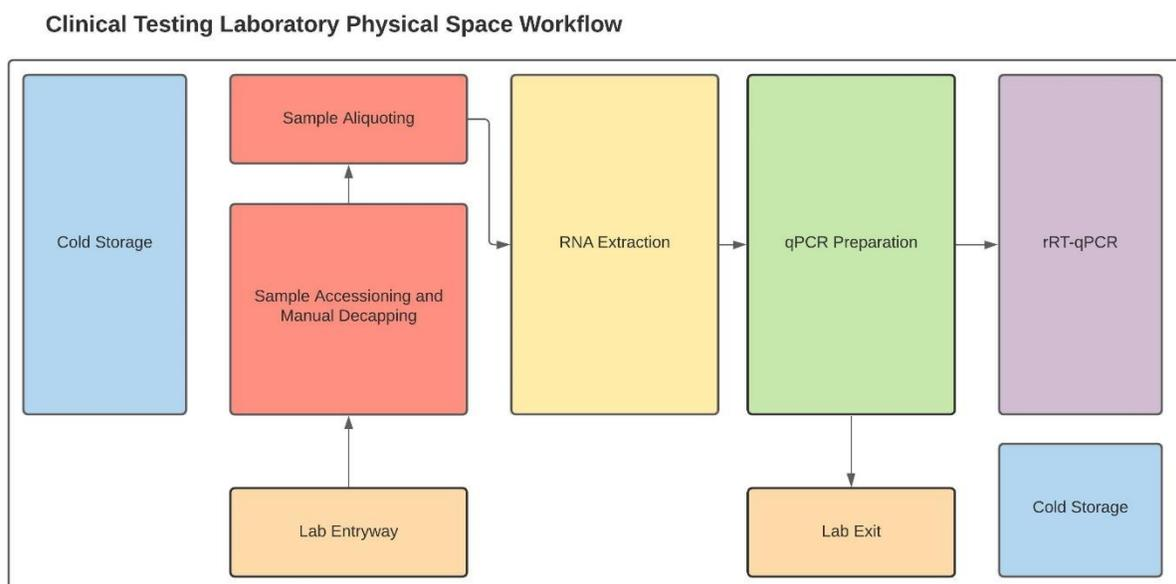
**Figure 3** The CTL workspace was divided into sections based on the tasks performed in each section: Sample Accessioning, Sample Aliquoting, RNA Extraction, qPCR Preparation, and RT-qPCR. Specific considerations were made to minimize cross contamination and to isolate the
