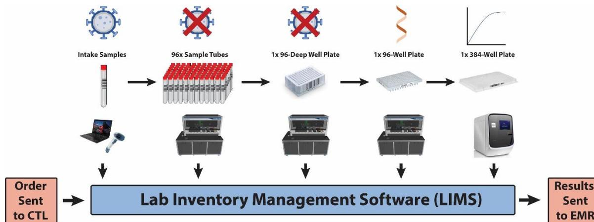
**Figure 6** The two EMR systems send test orders to the CTL for each individual sample. The LIMS integration utilizes APIs to transfer information related to the sample during the laboratory's testing process. This includes transferring information captured from each of the automation systems and the qPCR machine. The test results are reported out to the EMR systems through the LIMS.
