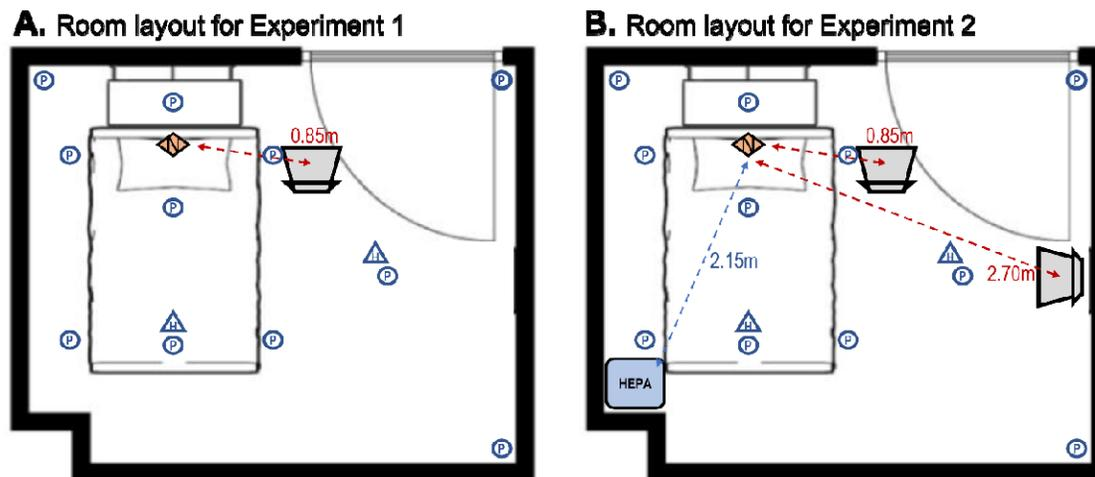
**Figure 1. Experimental layout for experiments 1 and 2.** All experiments were performed in a clinical room with dimensions  $4.0 \times 3.25 \times 2.7$  m (volume =  $35.1 \text{ m}^3$ ) containing a bed and one chair. Eleven settle plates (blue circles) were positioned identically between both experiments. Two hanging plates
