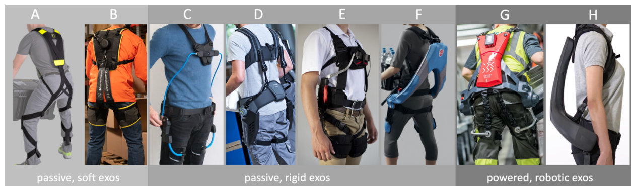
Figure 1. Examples of commercial back exos. Passive, soft exos (i.e., elastic exosuits made primarily from soft materials): A) Kinetic Edge Flex Lift, B) HeroWear Apex. Passive rigid exos (i.e., elastic exoskeletons made primarily from rigid components): C) Laevo, D) Ottobock Paexo Back, E) SuitX BackX, F) Innophys Muscle Suit Every. Powered robotic exos (i.e., using motors to assist): G) German Bionic Cray X, H) Atoun Model Y. Regardless of differences in componentry (rigid vs. soft) or actuation (passive vs. powered), each of these exos assists biomechanically by generating an extension moment (torque) about the lumbar spine during lifting, which reduces musculoskeletal loading on the user's low back.
