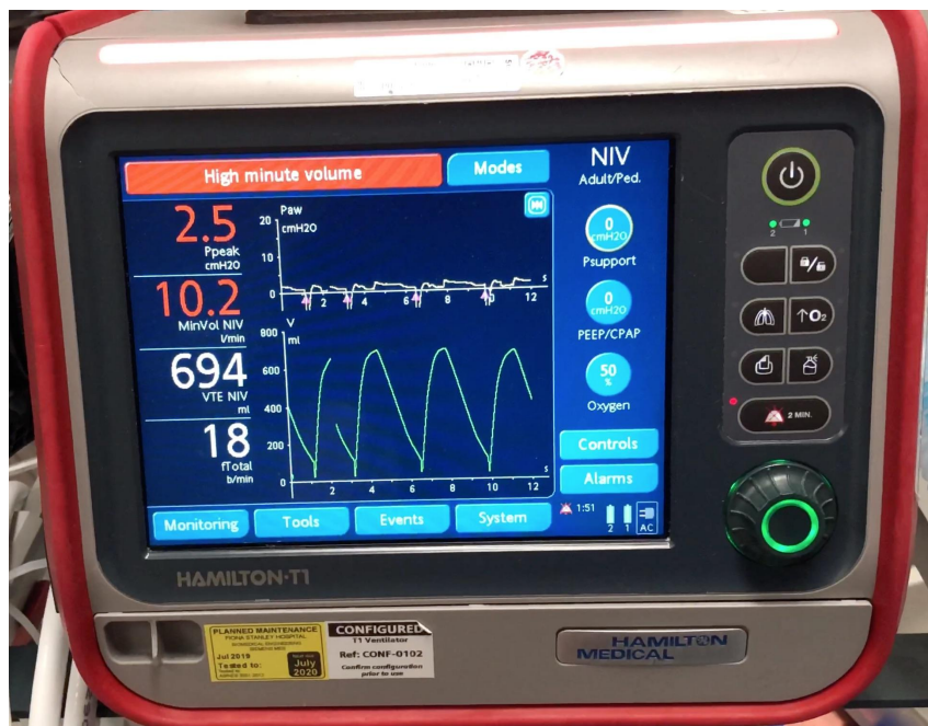
Volume waveform produced by NIGEL set to Vt 700ml, RR 18, during a trial of administering NIV to the lung simulator (current settings: zero support)
