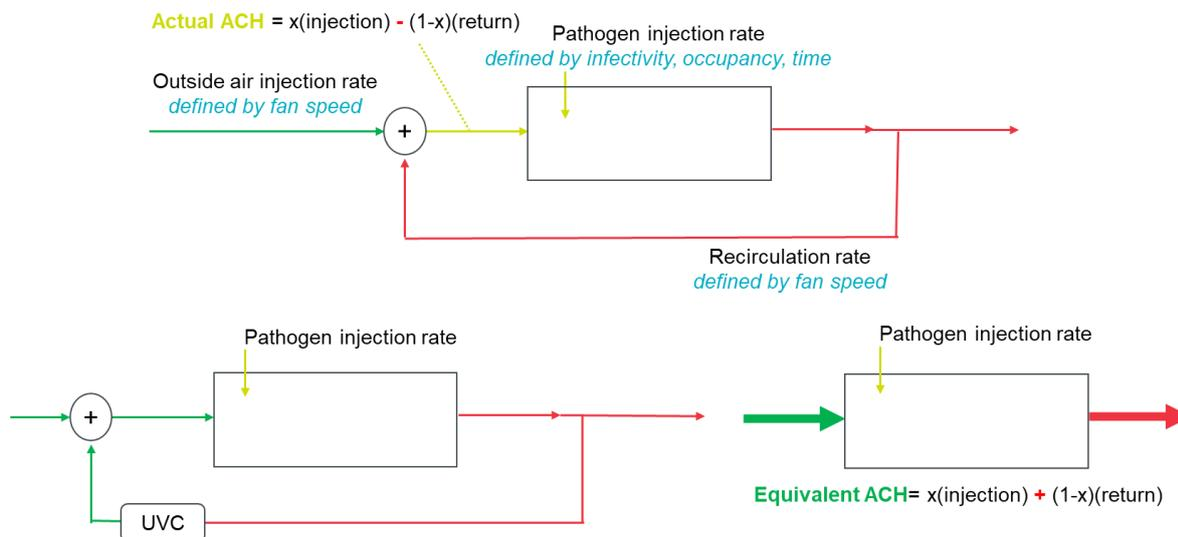
**Fig. 1:** Equivalent ACH (eACH) as it relates to fresh-air injection rate
