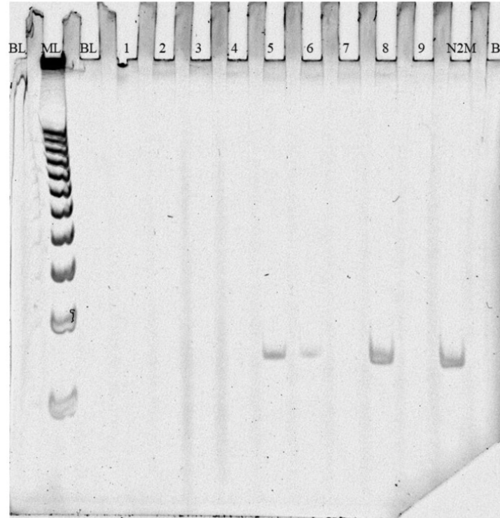
Figure 2. Example acrylamide gel image depicting all components indicative of a successful experiment. In this image, the first and last lanes labeled “BL” are negative controls loaded with nuclease-free water, and the lane labeled “ML” contains a 25 base pair ladder. IDT’s 2019-nCov’s specific N2 primer produces a PCR product that is 67 base pairs in length, seen in lane “N2M” for positive control purposes. Bands at the same location are considered to have tested positive for SARS-CoV-2, seen in lanes 5 and 6. These lanes contain the positive PCR product of experimental samples collected from stainless steel door handles to a student residence hall, as well as the university’s heavily populated Student Union.
