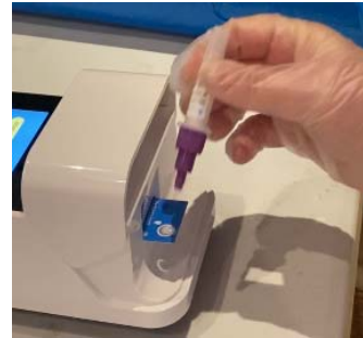
Fig. 2 The operator applies the extracted sample from the extraction vial onto the sample application area of the inserted test strip.
