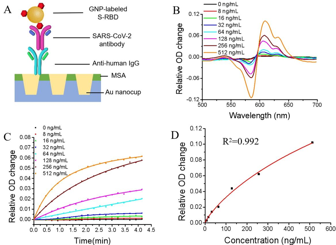
**Figure 2.** Label-free detection of the total SARS-CoV-2 NAs with colloidal GNP-enhanced NanoPISA. (A) Schematic diagram of the NanoPISA for the determination of SARS-CoV-2 NAs
