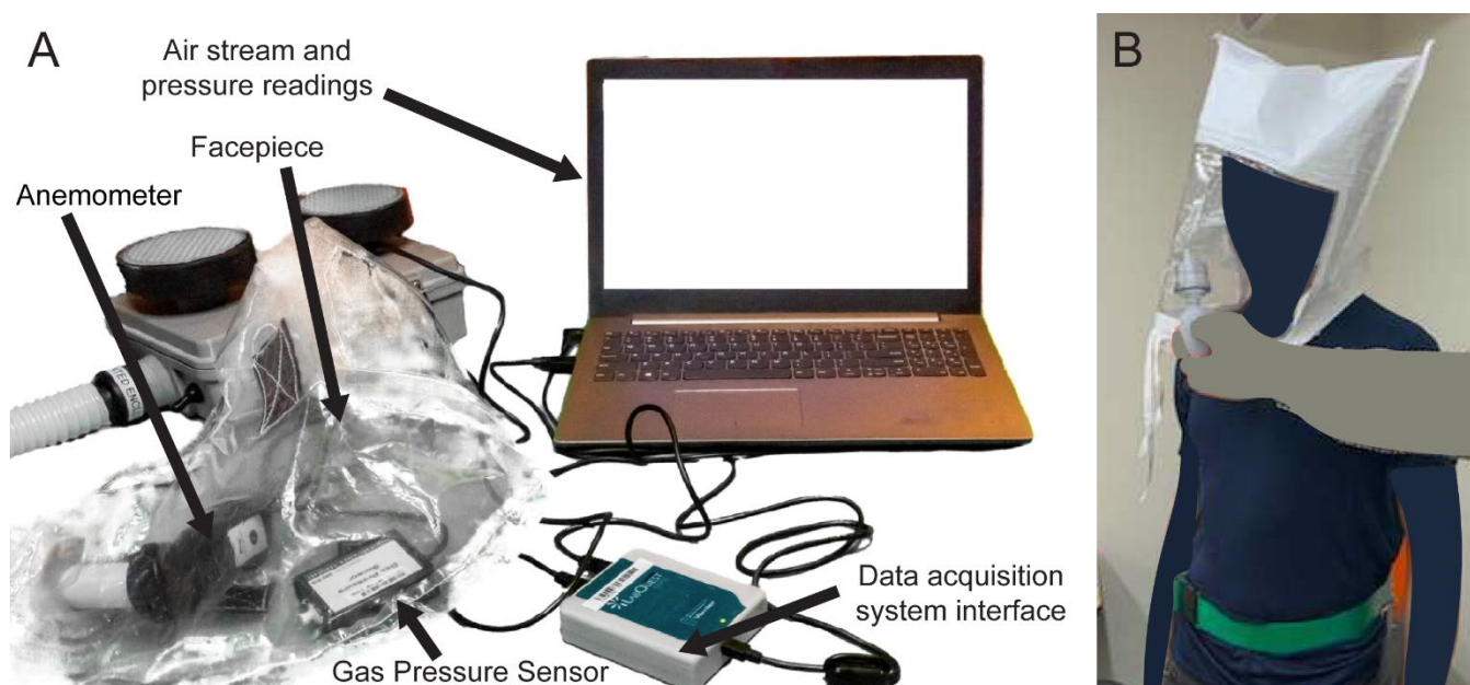
Figure 3: A) Test setup to measure flow rate and the positive pressure inside the facepiece, using Vernier Anemometer and Gas Pressure Sensor. PAPR facepiece contains anemometer and gas pressure sensor. Duck tape covers the neck opening of the facepiece for testing. B) Bitrex Fit Test setup.
