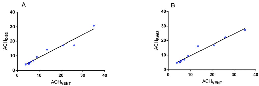
**Figure 4.** A: Correlations between ventilation rate by air flow ( $ACH_{VENT}$ ) and ventilation rates by time needed to reach 63% of excess  $CO_2$  generated using A: dry ice ( $ACH_{DI63}$ ) and B: baking soda and vinegar ( $ACH_{BV63}$ ).
