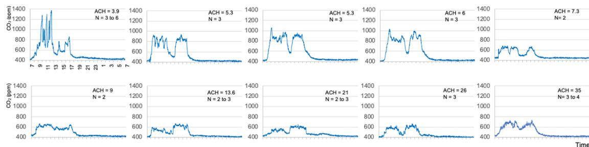
**Figure 2:** 24-hour continuous measurements of CO<sub>2</sub> levels in 10 dental treatment rooms with various ventilation rates. CO<sub>2</sub> accumulation occurred in rooms with lower ventilation rates (ACH ≤ 6). CO<sub>2</sub> levels stayed under 800 ppm in rooms with higher ventilation rate and lower number of persons. CO<sub>2</sub> level in nonworking hours is close to that of outdoor at 400 ppm in all the rooms.
