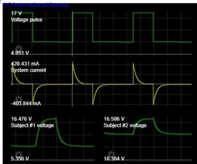
**Figure 3.** Records in a PCV simulation. All graphs show voltage or current as a function of time. Top: the voltage pulse generated by the "ventilator system". Medium: the current register in the system. Lower: the capacitor voltage that represents each subject, equivalent to the alveolar pressure in mechanical ventilation.
