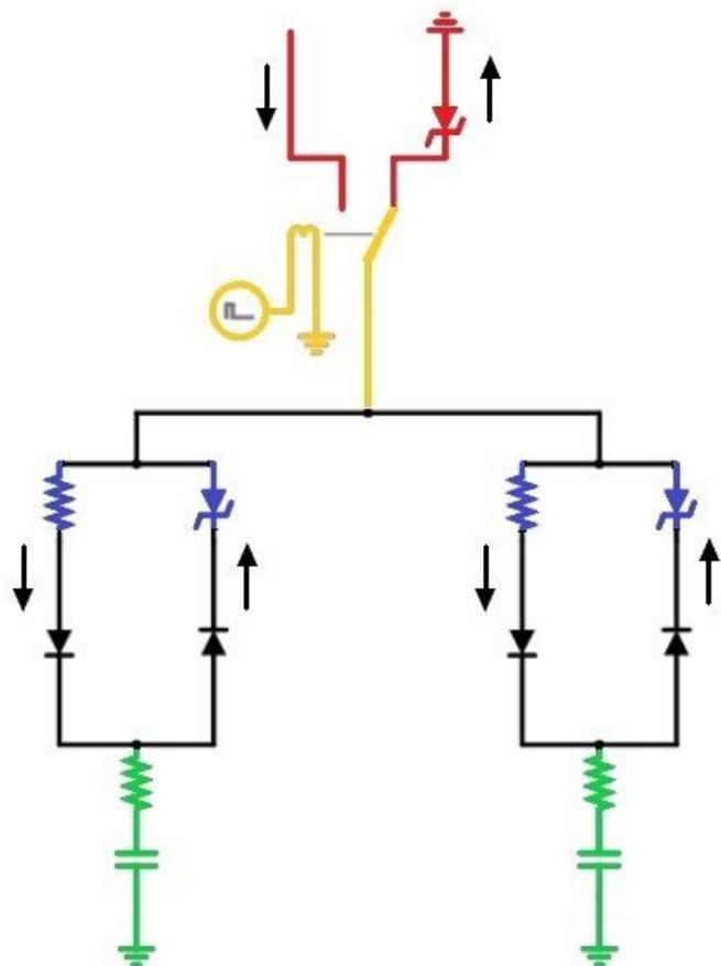
**Figure 2.** Electrical diagram of combined ventilation: in red, the "ventilator system"; in green, the "subject system"; in yellow, the connection between both systems through the relay; in blue, the DuplicAR system. The black arrows outside the circuit represent the direction of the current.
