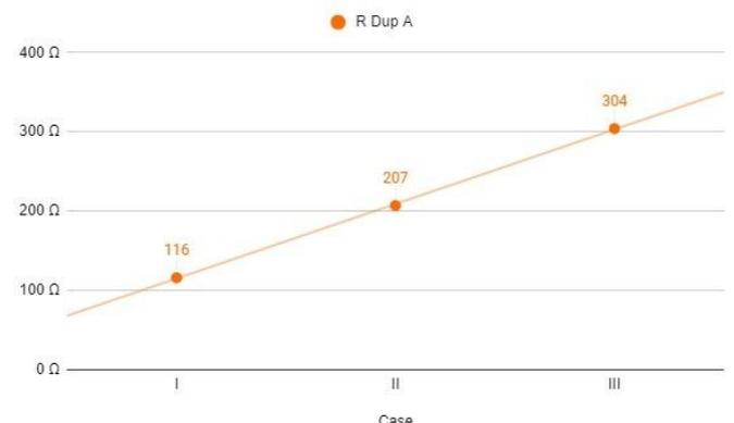
**Figure 13.** Stage 3 simulation, VCV mode. DuplicAR resistance of RC circuit A in each case.
