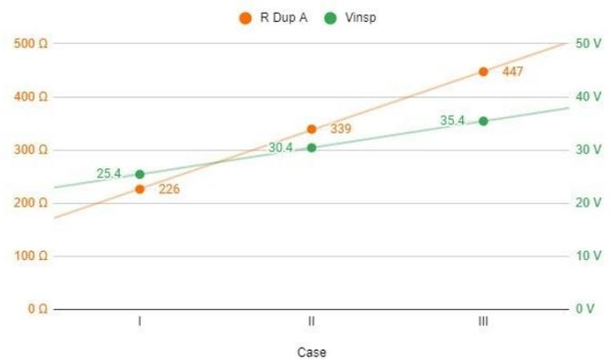
**Figure 12.** Stage 3 simulation, PCV mode. In green, power source voltage; in orange DuplicAR resistance of RC circuit A.
