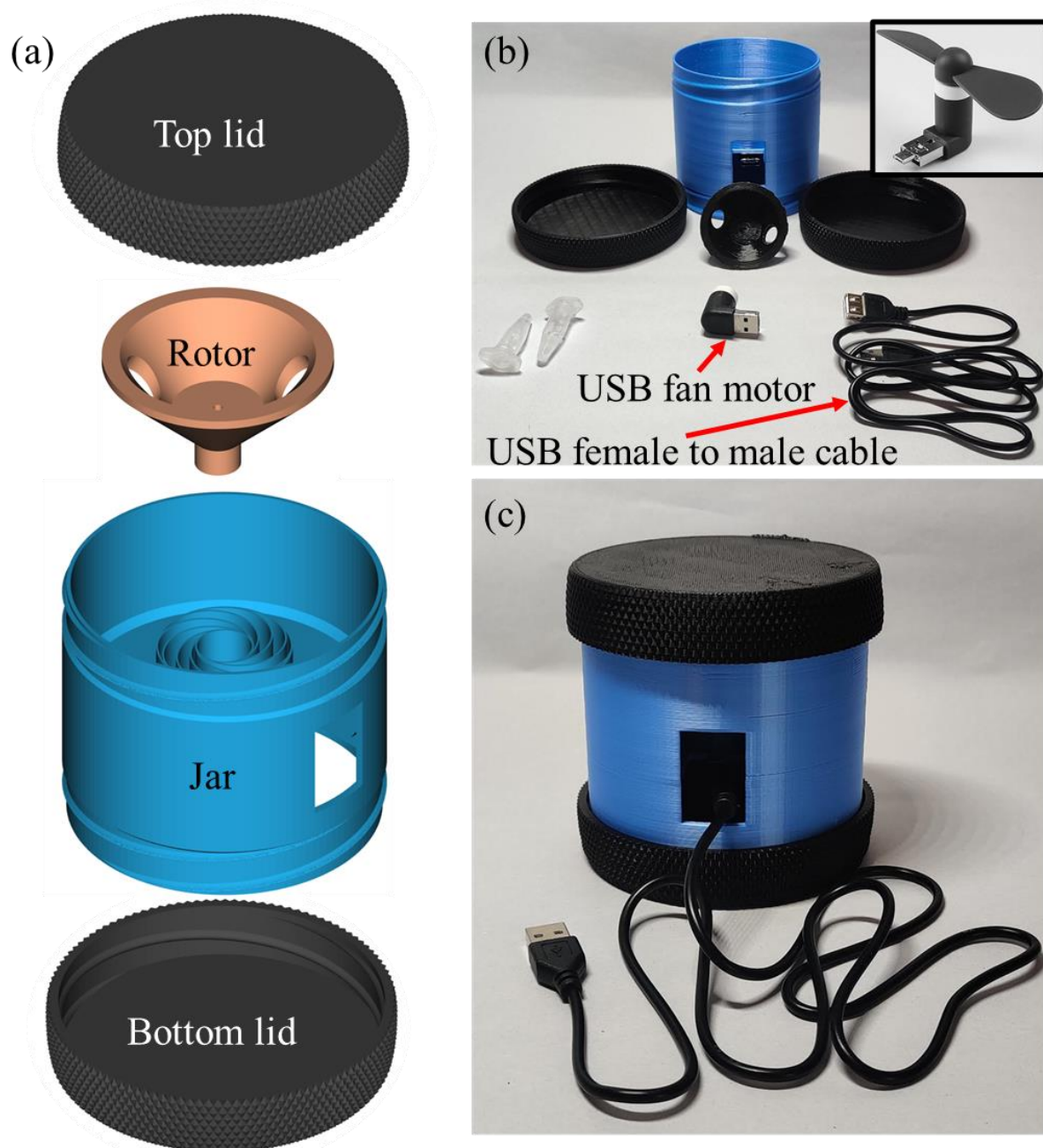
Figure 1: (a) CAD diagrams of 3D printed parts required for the Mobilefuge (b) The 3D printed parts and the electrical parts required to fabricate the Mobilefuge. The USB fan that powers the Mobilefuge is shown in the inset (c) Completely assembled Mobilefuge.
