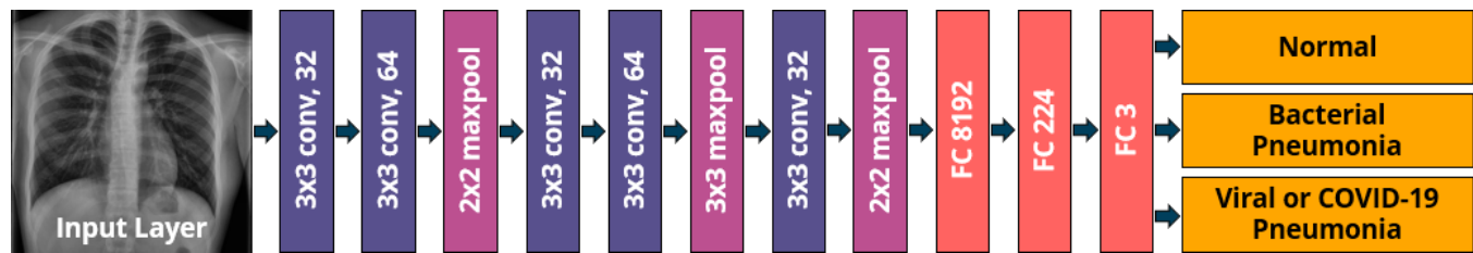
Figure 3: Architecture of the proposed CNN for pneumonia classification.
