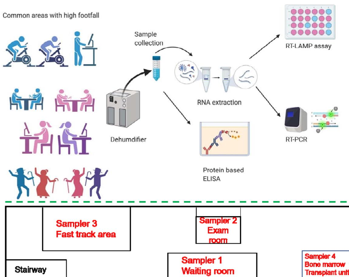
**Figure 1.** Schematic representation of sample collection and analysis for mass detection (top) and simplified layout of the hospital ward indicating the positions of various dehumidifiers during September 3-10, 2020 (bottom).
