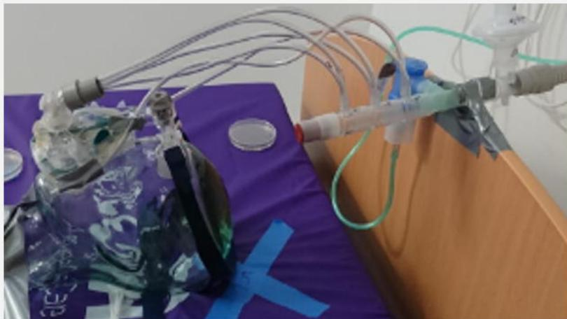
**E. Hood structure with HEPA filter**
