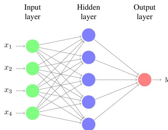
Fig. 1: Multilayer perceptron with one hidden layer
