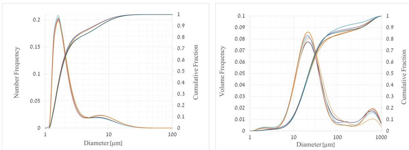
Figure 3. Spraytec measurements of number (left) and volume (right) size frequency and cumulative distributions of jet droplets, measured 30 cm from source. The different colors indicate different repetitions.
