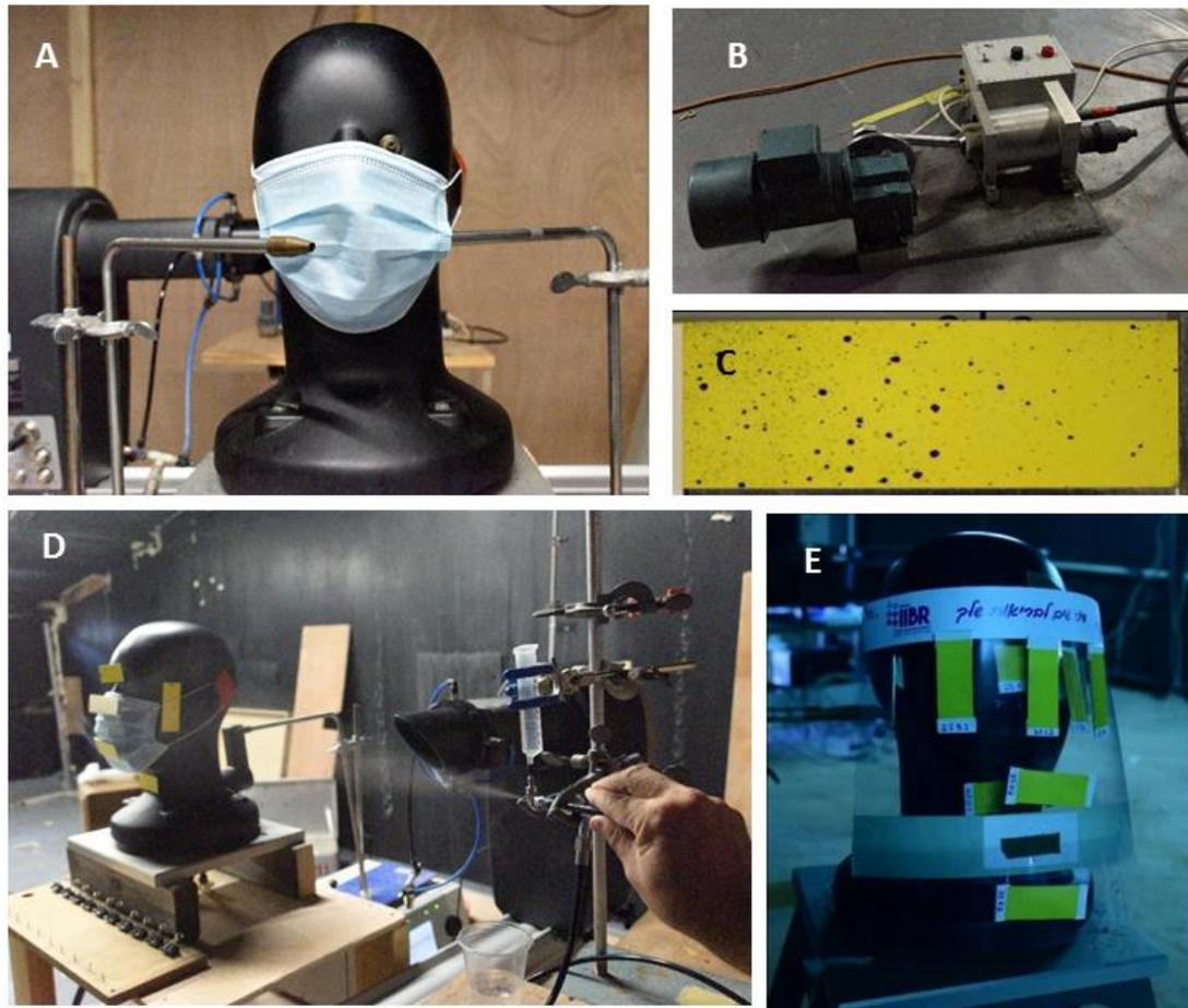
Figure 2. Elements of experimental setup. A) A manikin head with a fitted surgical mask. A probing tube for APS measurement is inserted through the right gap between the mask and the face. B) The breathing machine oscillatory pump. C) Water sensitive paper after exposure. D) A simulated expiratory event. The airbrush diffuser can be seen on the right. E) Water sensitive paper taped on the shield and on the manikin face underneath.
