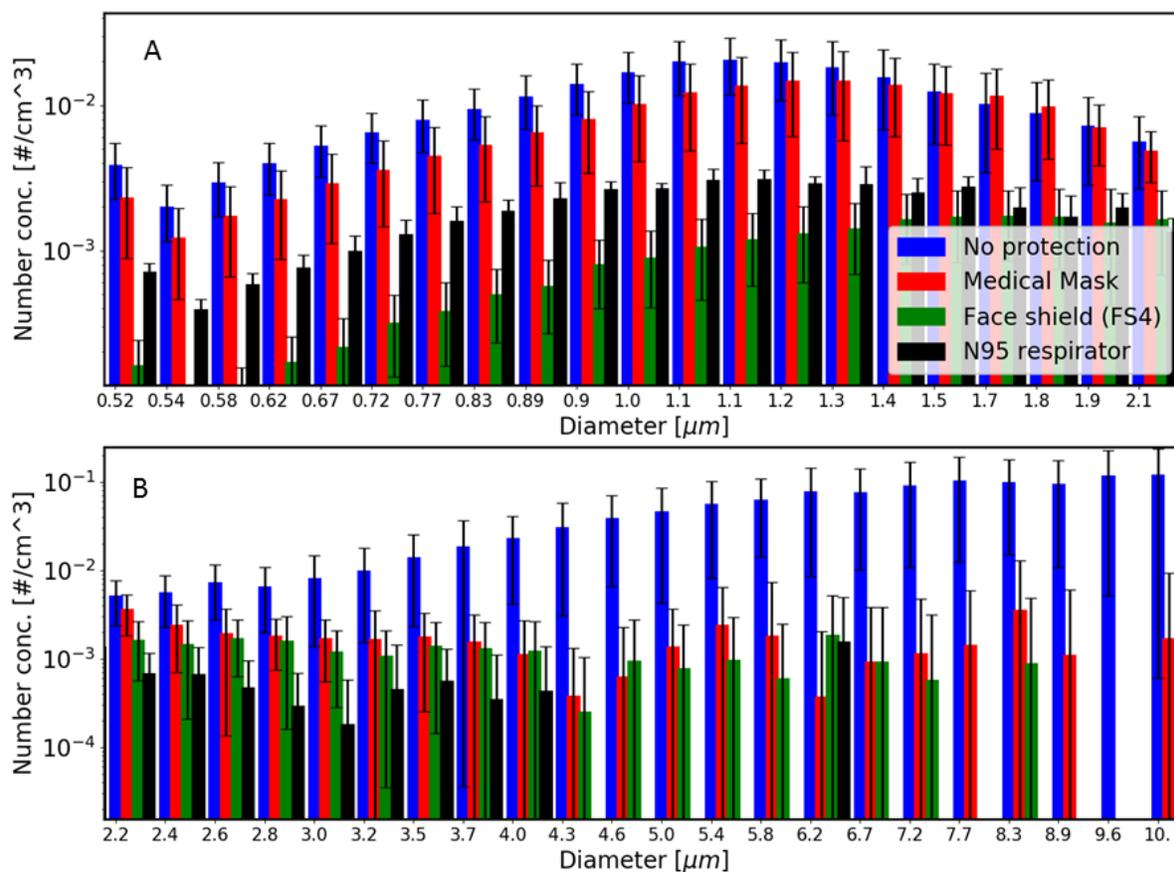
Figure 5. APS measurements statistics of inhaled particles number concentration, see Equation (2). The horizontal axis specifies the aerodynamic particle diameter (A- fine particles, B- large particles). Repetitions are grouped into four different cases as indicated by the different colors. The standard deviation among different repetitions in each group is indicated by error bars.
