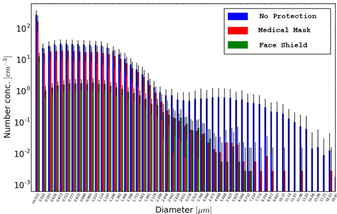
**Fig. 3: APS measurement statistics of inhaled particles Number concentration. The horizontal axis specifies the aerodynamic particle diameter. Repetitions are grouped into three different cases as indicated by the different colors. For each repetition, a single representative size distribution is taken at the moment of highest total number concentration. The bars reflect the average of different repetitions, and the variability between different repetitions is indicated by error bars.**
