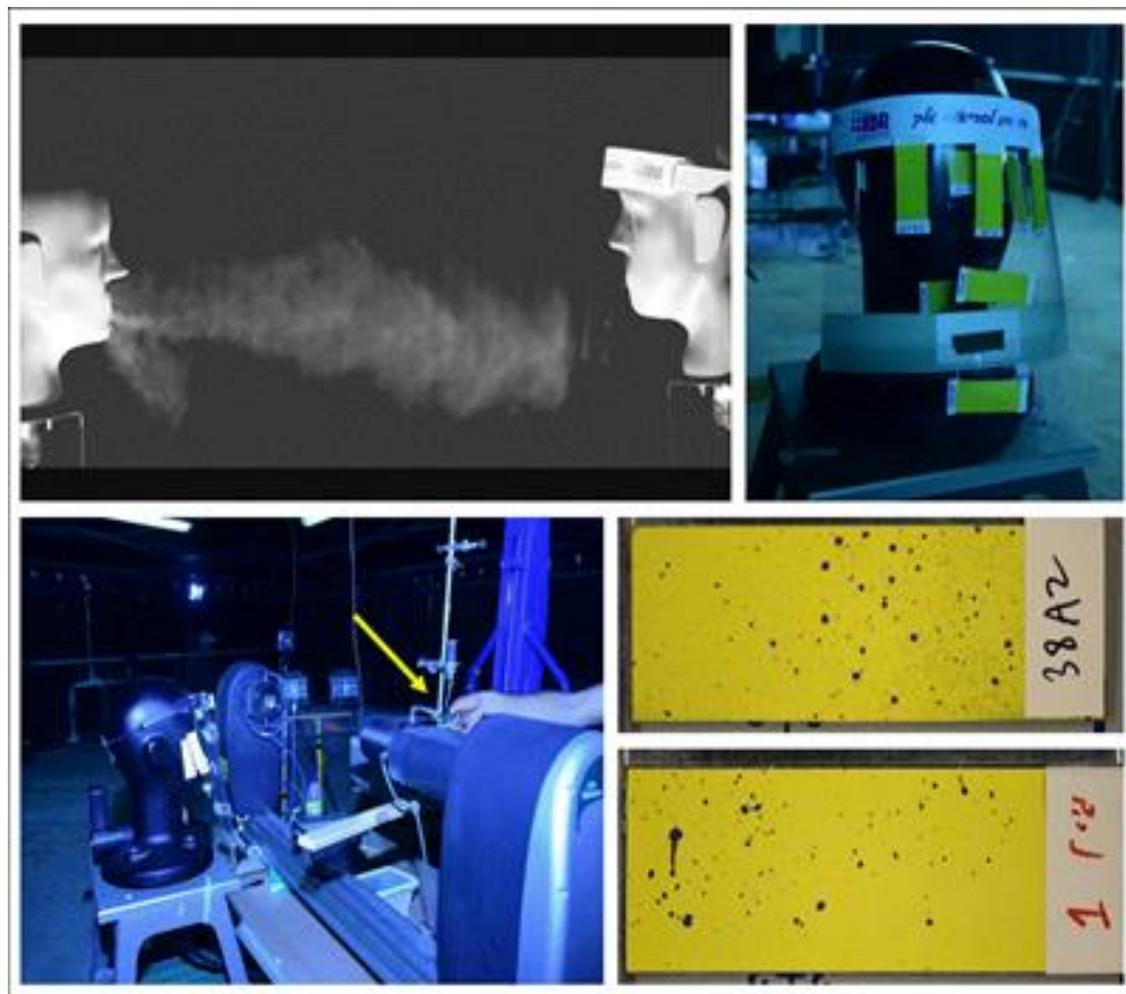
**Fig. 1: Experiment Setup.** Up left: diffuser was located behind the left manikin head, releasing the jet toward the right. Down left: An Airbrush diffuser (indicated by an arrow) is located facing the manikin head, while the “Spraytec” analyzer measures the droplet size distribution along the jet. Up right: Water sensitive papers taped on top of and below a face shield. Down right: Water sensitive papers marked by droplets stains of Airbrush spray (up) compared to real human sneeze (down).
