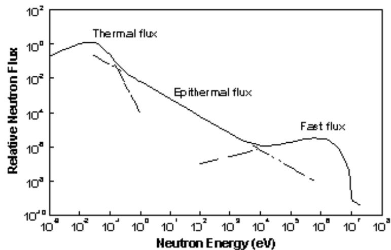
Figure 4: A typical reactor neutron energy spectrum showing the various components used to describe the neutron energy regions (Glascock, 2003).
