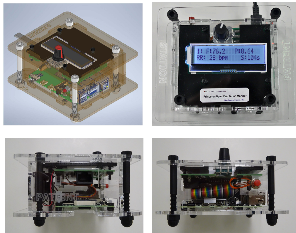
Fig 6. Interface box. Raspberry Pi based interface box sits at patient bedside. It provides an alarm system with a human interface and it relays sensor information to the central remote monitoring station.
