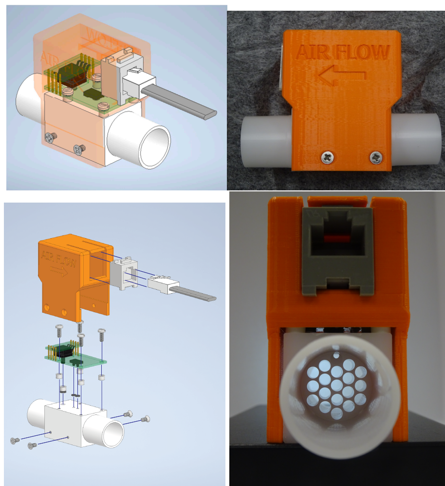
Fig 3. Flow-sensor assembly. A flow and pressure sensor are exposed to the flow element. The electronic sensor elements are mounted on circuit boards that connect to an external RaspberryPi controller via a standard RJ-45 jack.
