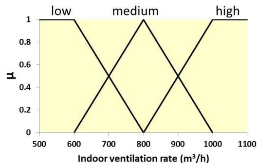
Figure 4. Membership functions of indoor ventilation rate.
