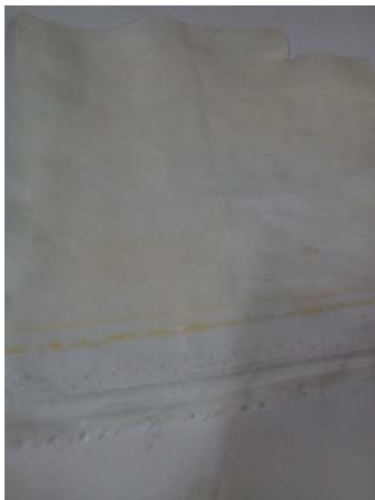
Photo 3: Cloth stained after repeated Hypochlorite treatment
