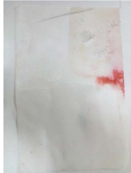
Photo 2: Cloth damaged after phenol treatment
