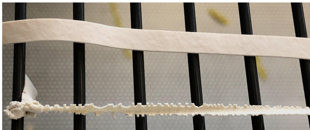
Figure S3. Example of strain-induced ozone damage (20 ppm, 30 minutes, 24°C, 38% RH) to bands separated from a Sperian N1125 respirator. ( Top ) Relaxed (not stretched) band underwent no visible damage and remained functional; ( bottom ) band tied off at 2.4 times its relaxed length during ozone exposure failed.
