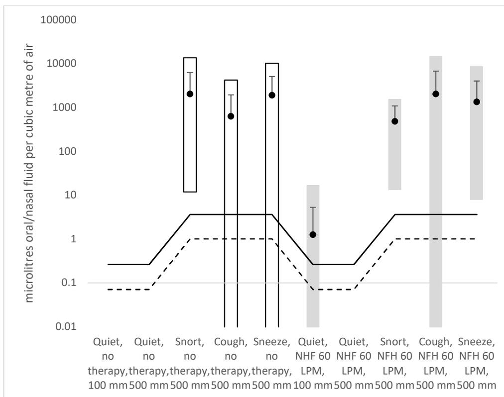
**Figure 4: Summary of data from chemical marker test. Black circles are the means, error bars are +/- one standard deviation (due to the logarithmic scale, the negative error bar is obscured by the datapoint marker), and bars show the range from minimum to maximum. White bars are no therapy, grey bars are 60 LPM NHF. The solid line is the maximum detectability limit and the dashed line is the minimum (as detectability depends on air flow rate).**
