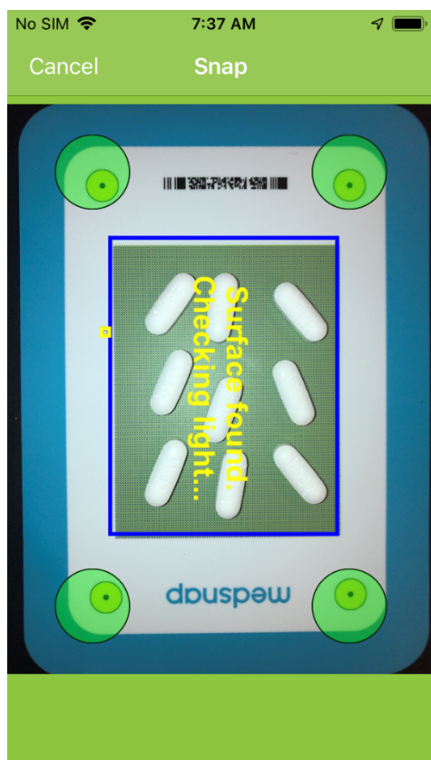
Figure 2. MedSnap DA and VR guide the user to properly align the camera with the Snap Surface then automatically take an image
