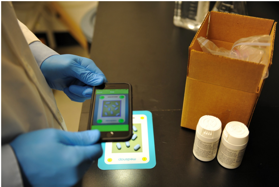
Figure 1. Use of the MedSnap VR application to test a sample of tablets to determine authenticity. The vinyl Snap Surface is used as a background for the sample.
