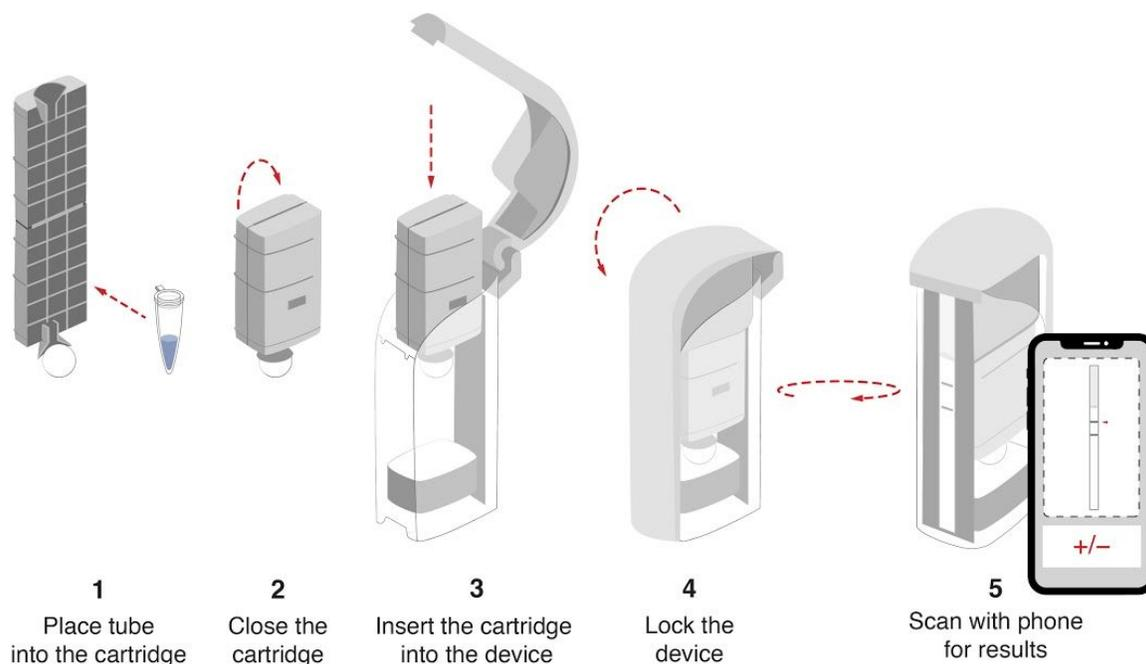
**Figure 6: Device cartridge for reading out the STOPCovid test.** In order to limit amplicon spread and contamination, sealed reaction tubes are placed in detection cartridges (Ustar, <http://www.bioustar.com/en/about.aspx>). User closes the cartridge and pulls the handle to release reaction onto a lateral flow strip. A mobile phone application can be used for quantitating the band intensity and determining the test result.
