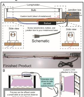
Figure 3: A) Schematic and finished product of the custom fixture that can be easily created to fit an existing UV-C bulb from a BSC. This custom fixture is one of the options depending on the end-user circumstances. The UV-C output should be measured using a UV-C meter for each configuration individual of sterilization set-up to determine the appropriate irradiation time. B) UVGI devices can be arrayed in a medical setting by affixing to available items such as tables or IV poles.
