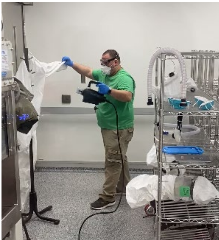
Supplementary Figure 1: Illustrative photograph of handheld device processing before sterilization by environmental SteraMist system, on a DuPont Tyvek® 400 coverall.
