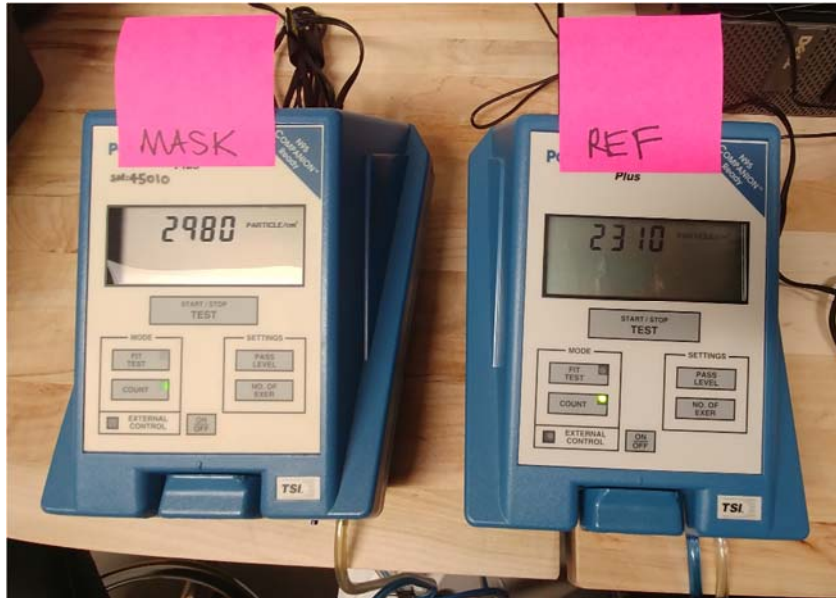
Figure 1. Testing set up included two TSI PortaCount Plus Model 8028 instruments sampling concurrently in Count Mode. The PortaCount labeled “Mask” was used to sample air inside the masks, while the PortaCount labeled “Ref” was used to sample air just outside the mask.
