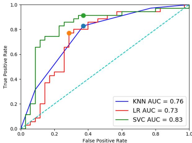
**Fig. 5.** Receiver operating characteristic curves for the three classifiers evaluated in this work for cyanosis detection. The filled circles represent the operating points resulting in the other performance statistics. (Small differences exist due to the leave-one-out cross-validation approach.)
