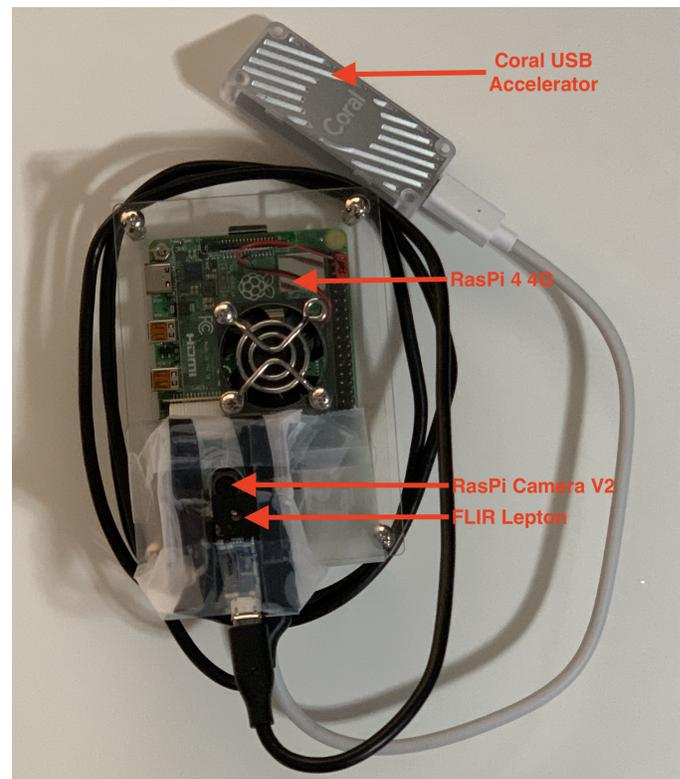
**Fig. 1.** Left: Hardware configuration consisting of a Raspberry Pi 4 (4 GB RAM), a Google Coral USB accelerator (top), a RasPi Camera v2 and a FLIR Lepton 3.5 Radiometry Long-Wave Infrared Camera. Right: Installation of system with all cabling including power and external monitor for visualization (not shown or needed for detection).
