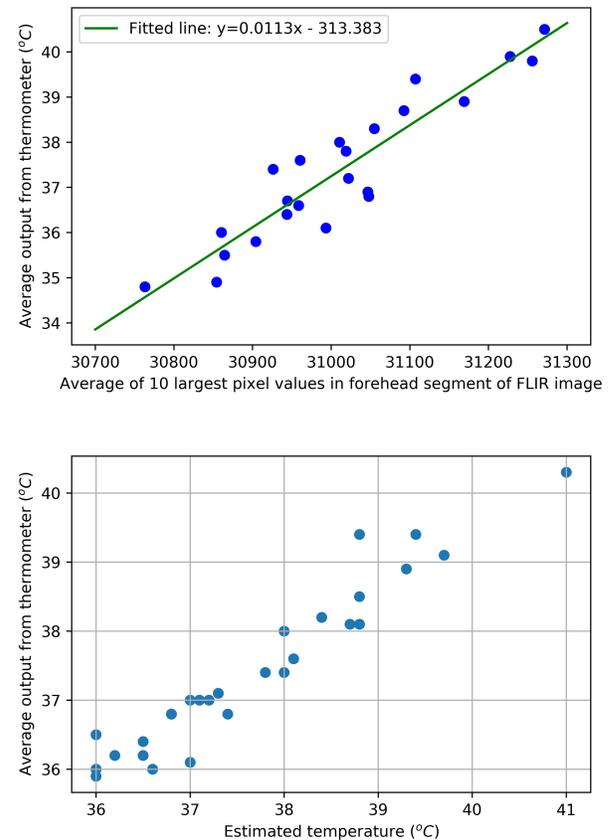
**Fig. 4.** Upper: Calibration of FLIR images using a bottle of water: Best fitted line between the average temperature from the thermometer and the FLIR pixel values had a root mean square error (RMSE) of 0.57 °C. Lower: Estimated temperature vs. temperature measured from thermometer. The Pearson correlation between the parameters was found to be 0.96 and the RMSE difference between them was 0.41 °C.
