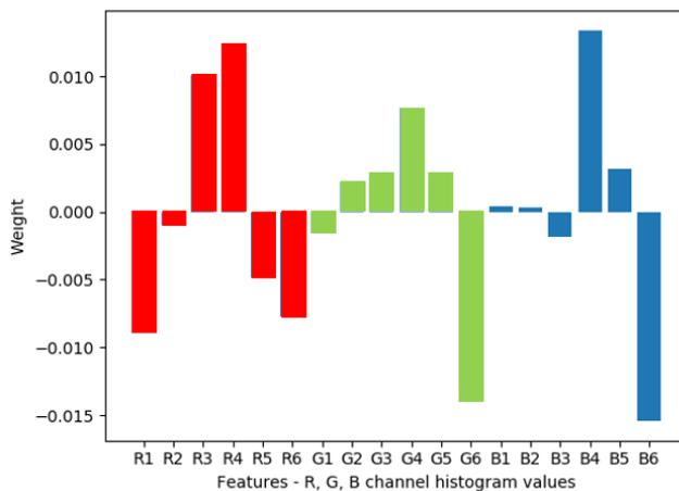
**Fig. 6.** Weighting of features from logistic regression. The features are the histogram values the R, G and B channels. Positive coefficients refer to cyanotic condition and negative refer to non-cyanotic.
